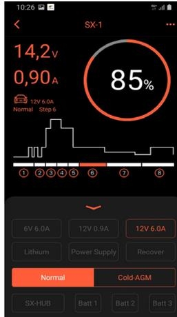
To start the charging process, select the desired charging mode (6V, 12V-0.9A, 12V-6.0A, Lithium, Power Supply or Recover).
