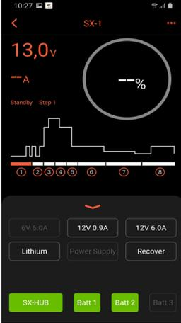
Connect the switcher SX-HUB to the charger and at least one battery to enable the switcher on the app ("SX-HUB" button become green).
