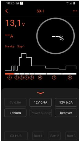
On this page you can start the charging process and see all the battery data: voltage, current, charging percentage and actual charging phase.
