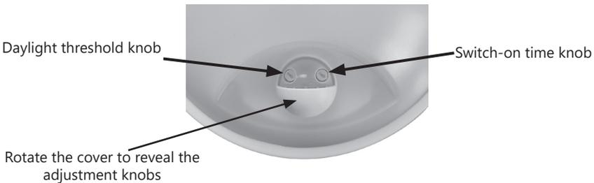
1. Rotate the cover that hides the PIR sensor adjustment knobs.
