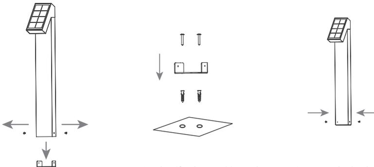
1. Detach the fixing bracket at the bottom of the floodlight by unscrewing the two lateral fixing screws.
