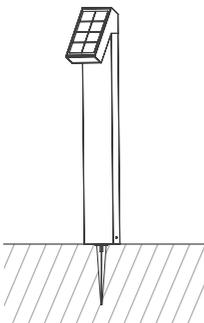
1. Screw and secure the ground stake to the floodlight.
